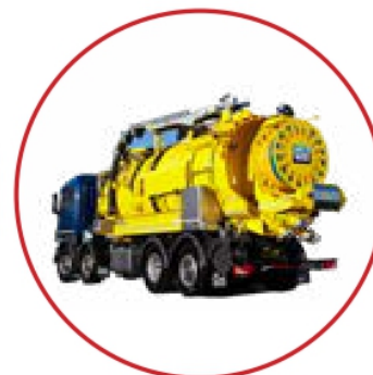
Vehicles equipped for water jetting
