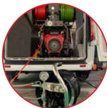
domestic drains and condominal sewer cleaning units
